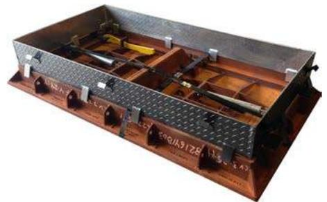
Available forming skirt simplifies precasting the hatch in concrete—no need for added forming to protect the inner hatch. The leave-in-place aluminum skirt can be made to fit any concrete slab thickness. (Image showing hatch upside down with forming skirt.)
