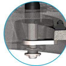
The cam lock provides improved security to frame and cover assemblies, and also eliminates loose and missing fasteners. The cam lock wrench is only removable when the cover is in the locked position, ensuring it is engaged.
