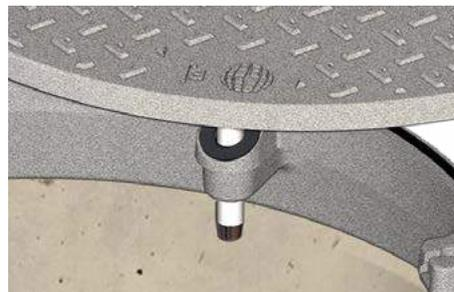
To open the cover, slightly lift, and rotate the cover. The patented design provides cover lift and rotation with minimal effort. Worker safety is improved by eliminating the need to hoist heavy covers when opening or closing the elevated unit.
