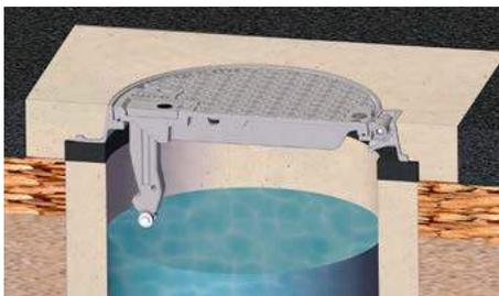
Illustrating the STORMSURGE® Access Assembly in the closed position.
