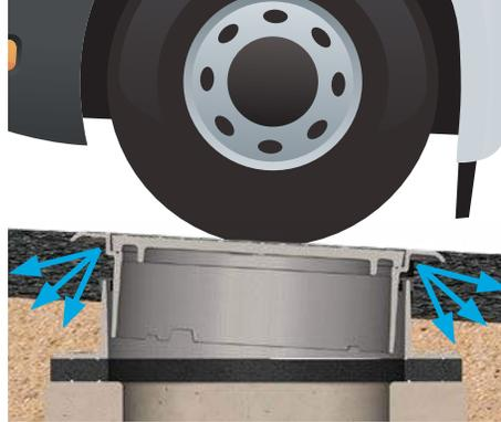
Once installed, the unit will continue to move with the road surface. The road surface aids in absorption of traffic vibration and shock, further protecting the life of your infrastructure and critical underground structures.
