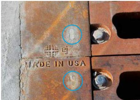
Venting slots in the frame rail allow for air to escape during the pouring process, fully filling the voids with concrete for support and weight disbursement.
