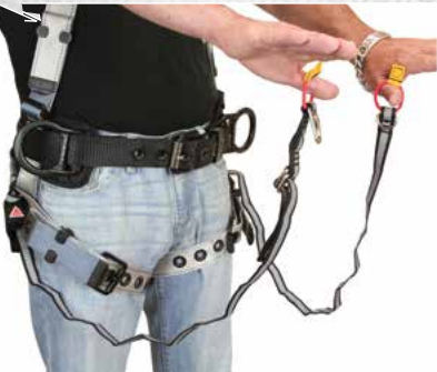
Pull red loops forward to release pack closure and deploy the full length of the reflective straps.
